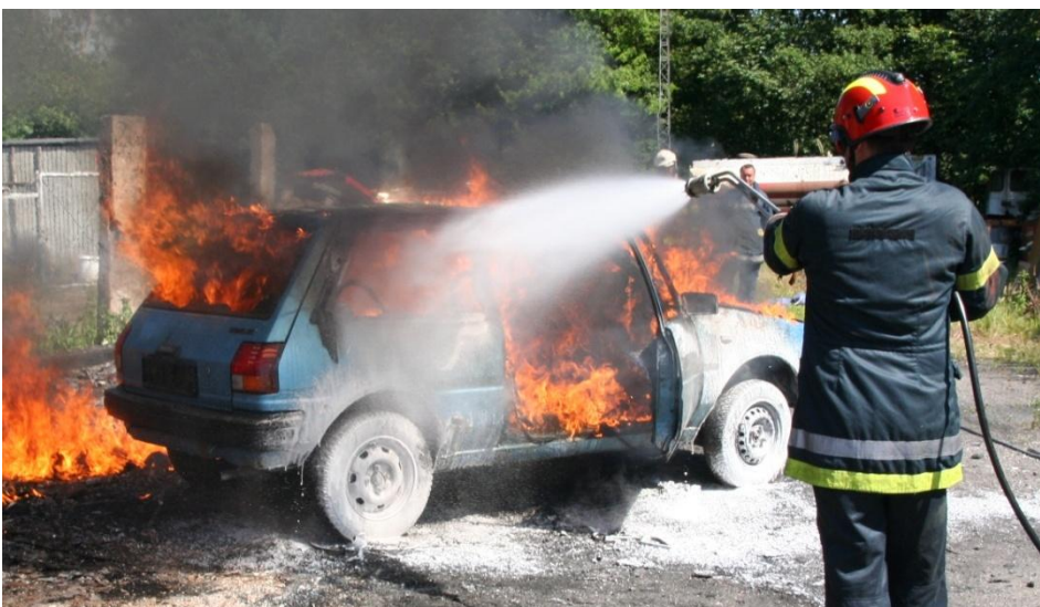
A car fire extinguished with 15 litres of water and foam
