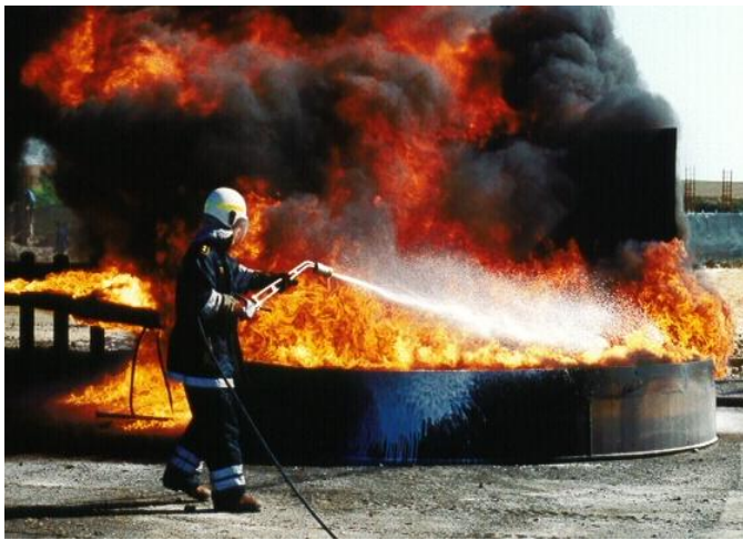
A 500 litres jet fuel fire extinguished with 38 litres
